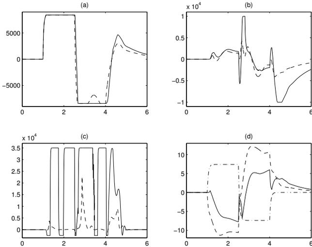
Fig. 4. (a)  $F_{y,f}$  with the controller  $C_{sm}$  (solid),  $F_{y,f}$  with the controller  $C_w$  (dashed) [N vs s]; (b)  $M_z$  with the controller  $C_{sm}$  (solid),  $M_z$  with the controller  $C_w$  (dashed) [Nm vs s]; (c)  $b_x$  with the controller  $C_{sm}$  (solid),  $b_x$  with the controller  $C_w$  (dashed) [m rad/s vs s]; (d)  $\delta_c$  with the controller  $C_{sm}$  (solid),  $\delta_c$  with the controller  $C_w$  (dashed),  $\delta_d$  (dash-dot) [deg vs s]
