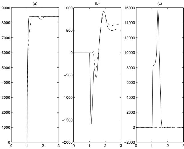
Fig. 2. (a)  $F_{y,f}$  with 3 actuators (solid),  $F_{y,f}$  with 2 actuators (dashed) [N] vs time [s]; (b)  $M_z$  with 3 actuators (solid),  $M_z$  with 2 actuators (dashed) [Nm] vs time [s]; (c)  $b_x$  with 3 actuators (solid),  $b_x$  with 2 actuators (dashed) [Nm-rad/s] vs time [s]
