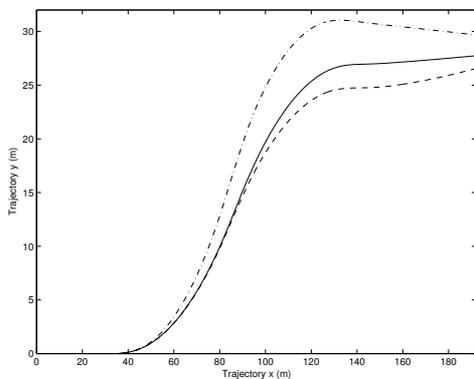
Fig. 6. Trajectory in the plane: reference (dash-dot), trajectory with the controller  $C_{sm}$  (solid), trajectory with the controller  $C_w$  (dashed)
