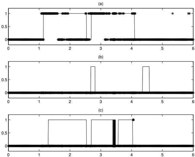
Fig. 5. Actuator saturation (1) or out of saturation (0) vs time [s], in the case of the controller  $C_{sm}$  (solid) or with the controller  $C_w$  (stars): (a)  $\Delta F_{y,f}$ ; (b)  $M_z$ ; (c)  $b_x$
