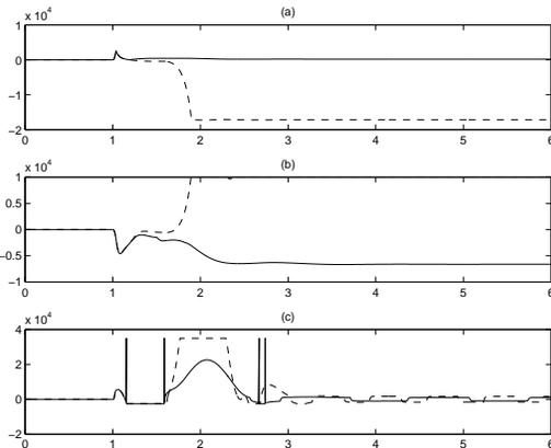
Fig. 5. (a)  $F_{y,f}$  with limiting function and variable reference (solid),  $F_{y,f}$  with linear saturation function (dashed) [N] vs time [s]; (b)  $M_z$  with limiting function and variable reference (solid),  $M_z$  with linear saturation function (dashed) [Nm] vs time [s]; (c)  $b_x$  with limiting function and variable reference (solid),  $b_x$  with linear saturation function (dashed) [Nm rad/s] vs time [s]
