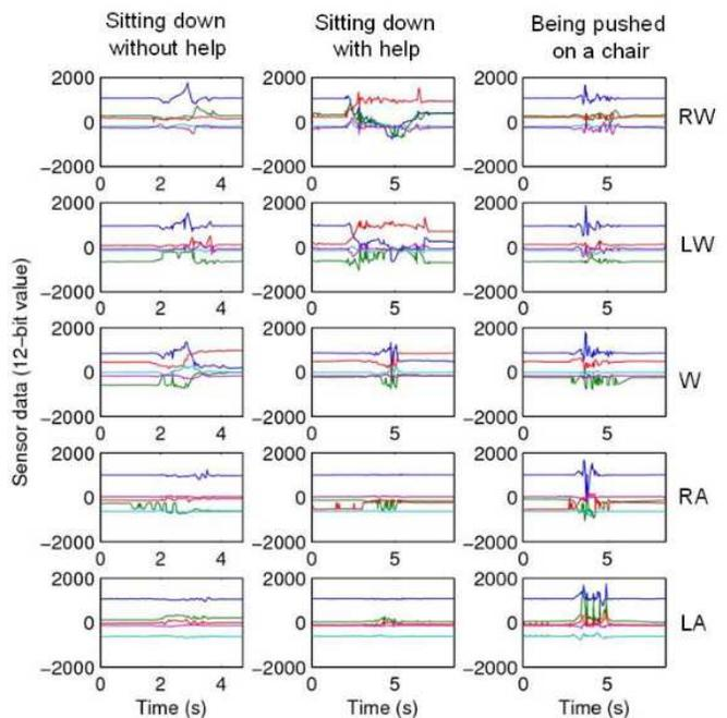
**Figure 6.** Sensor outputs for the action of sitting down in three situations.
