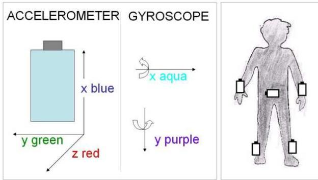
**Figure 3.** Meaning of the different colors that appear in the sensor readings and position of the body sensors.
